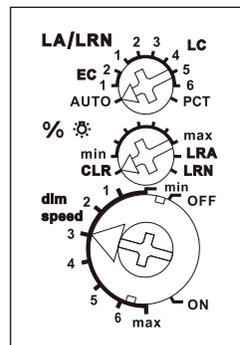
The upper rotary switch LA/LRN is first required for teach-in and defines in operation whether automatic lamp detection should be activated or special comfort positions:
