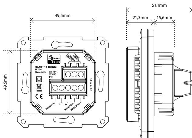
To be able to read the Power Metering, the load needs to be connected to both heating L + N.
