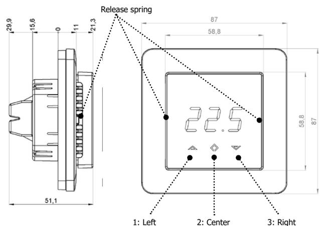
Use e.g. a small slotted screwdriver. Start by carefully removing the front cover by pushing the release springs. The front cover and the frame can now be removed.
